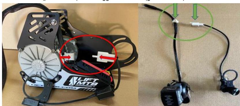
**For models before August 2020** the operation remains the same, simply the wiring changes for this it will be necessary to connect the connector of the sensor in series on the trigger connector (yellow arrows on the photo).
