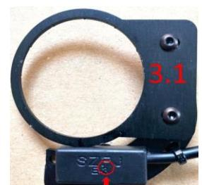
**ATTENTION:** The zone where the sensor detects the movement is located at the height of the "F" of the writing "SZFJ" (photo 3.1) this letter must be placed as close as possible to the axis, any reversal of position of any of the items will cause a malfunction.
