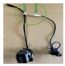
For models before August 2020 the operation remains the same, simply the wiring changes for this it will be necessary to connect the connector of the sensor in series to the trigger connector (yellow arrows in the photo).
